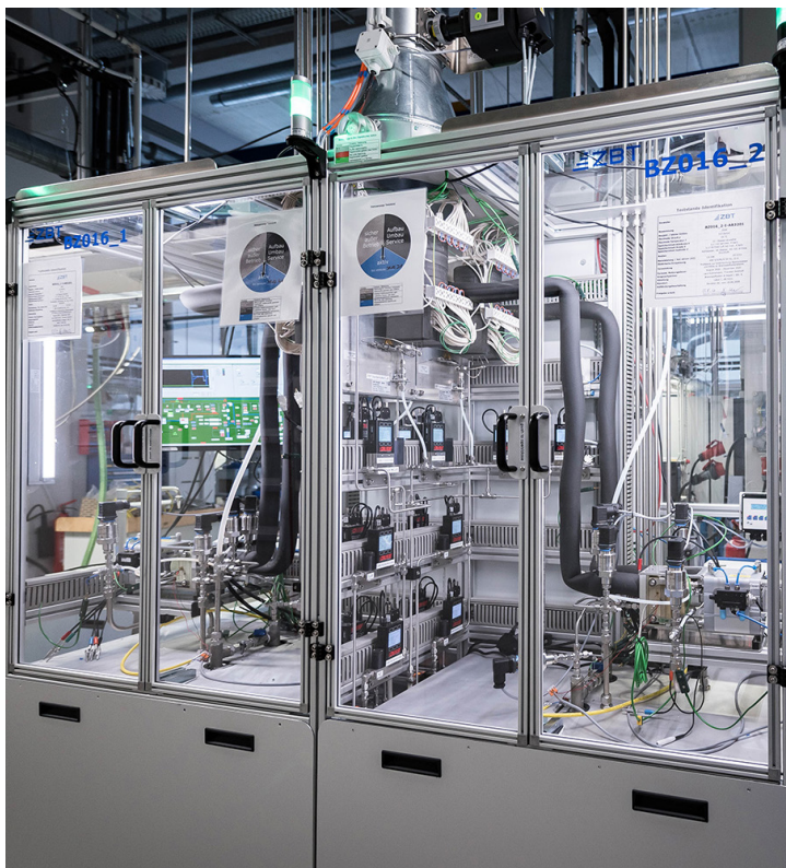
Figure 5. The process volume downstream of the flow controller was decreased after the device was optimized, resulting in a slower flow control response.
