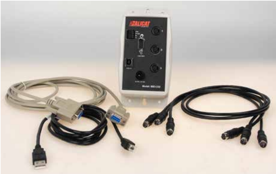
Although serial communications are normally one data stream to one comport, accessories like Alicat’s multidrop box permit up to 26 serial instruments to use a single computer comport or PLC connection. This allows for greater complexity of systems controlled by serial communications.
