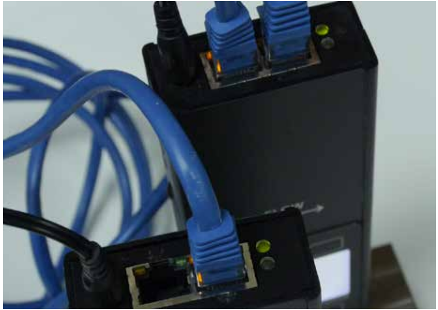
Device level ring connections for Ethernet/IP devices.
