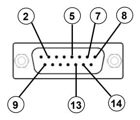
**Note:** The above pin-out is correct for units with a **DB15K** pin-out. If your unit is marked **DB15** or **DB15H**, you must use the correct pin-out (see pages 1 and 2).
